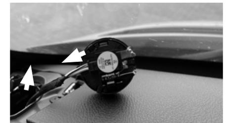
In the next step, lever the original tweeter out of its holder. Here you should carefully unclip the tweeter with a suitable pointed lever tool and lever it upwards. Then remove the original connection cable of the tweeter.
